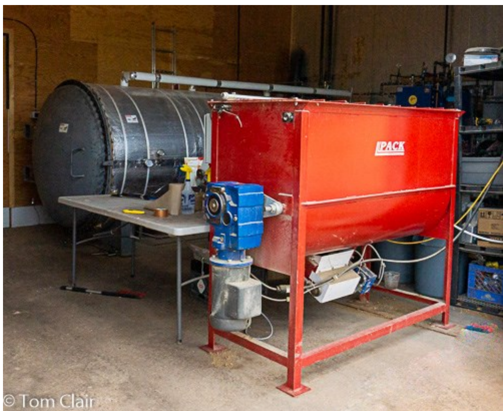
Figure 4. Wood chip sterilizing and fertilizing equipment.
